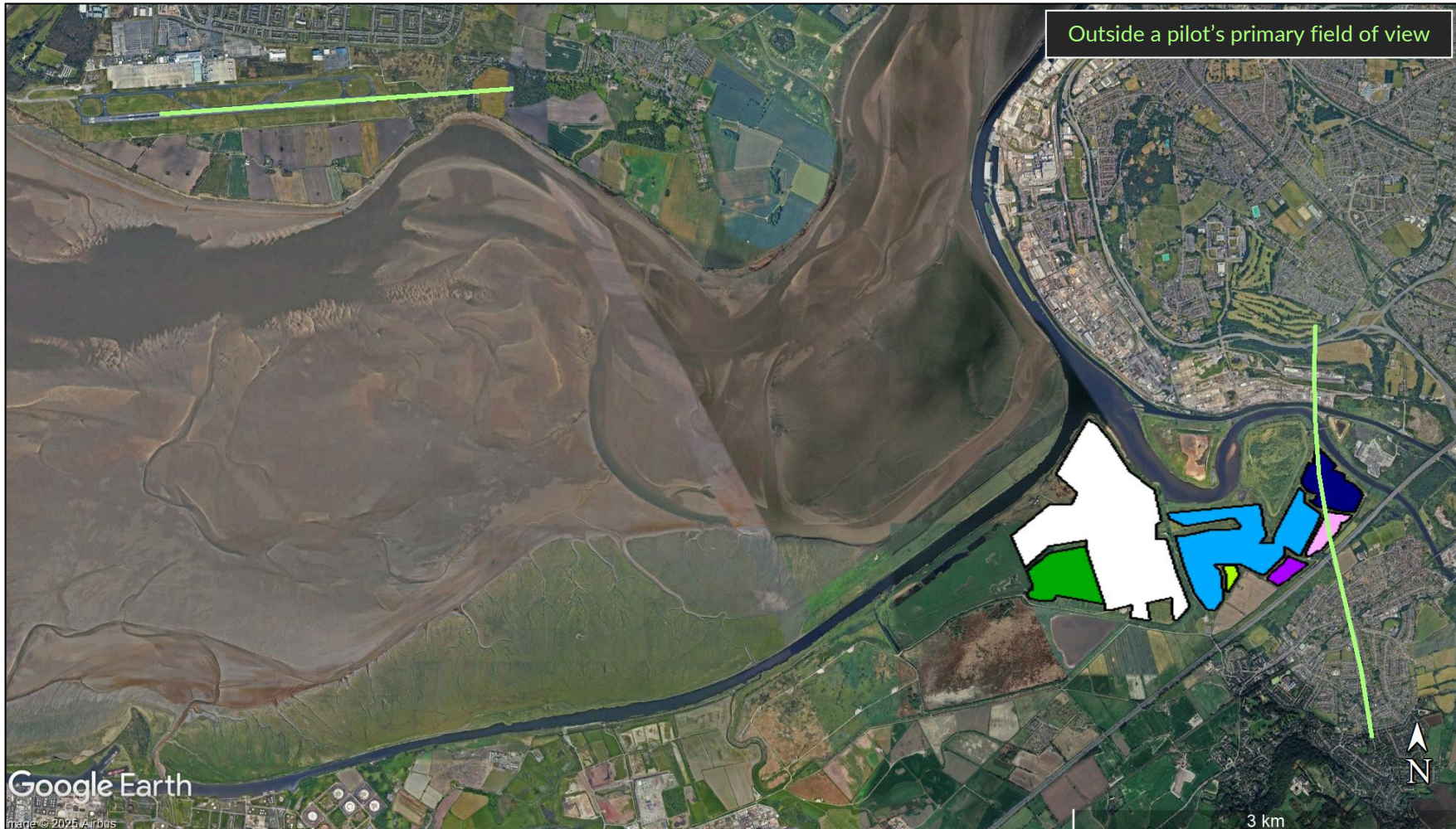
Figure 19 Solar reflections towards commercial visual approach
