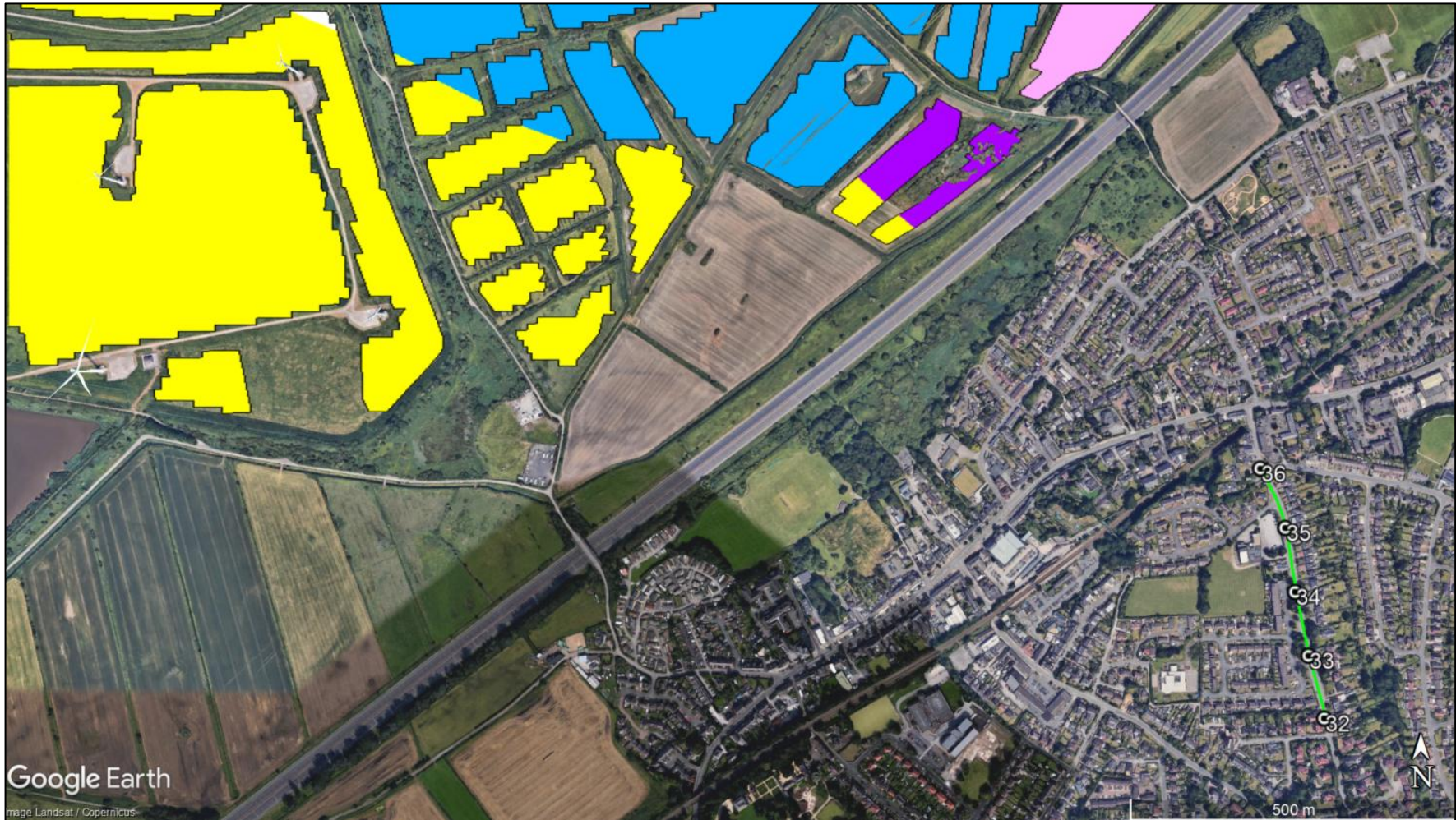
Figure J37 Reflecting panel areas for road receptors 32 to 36
