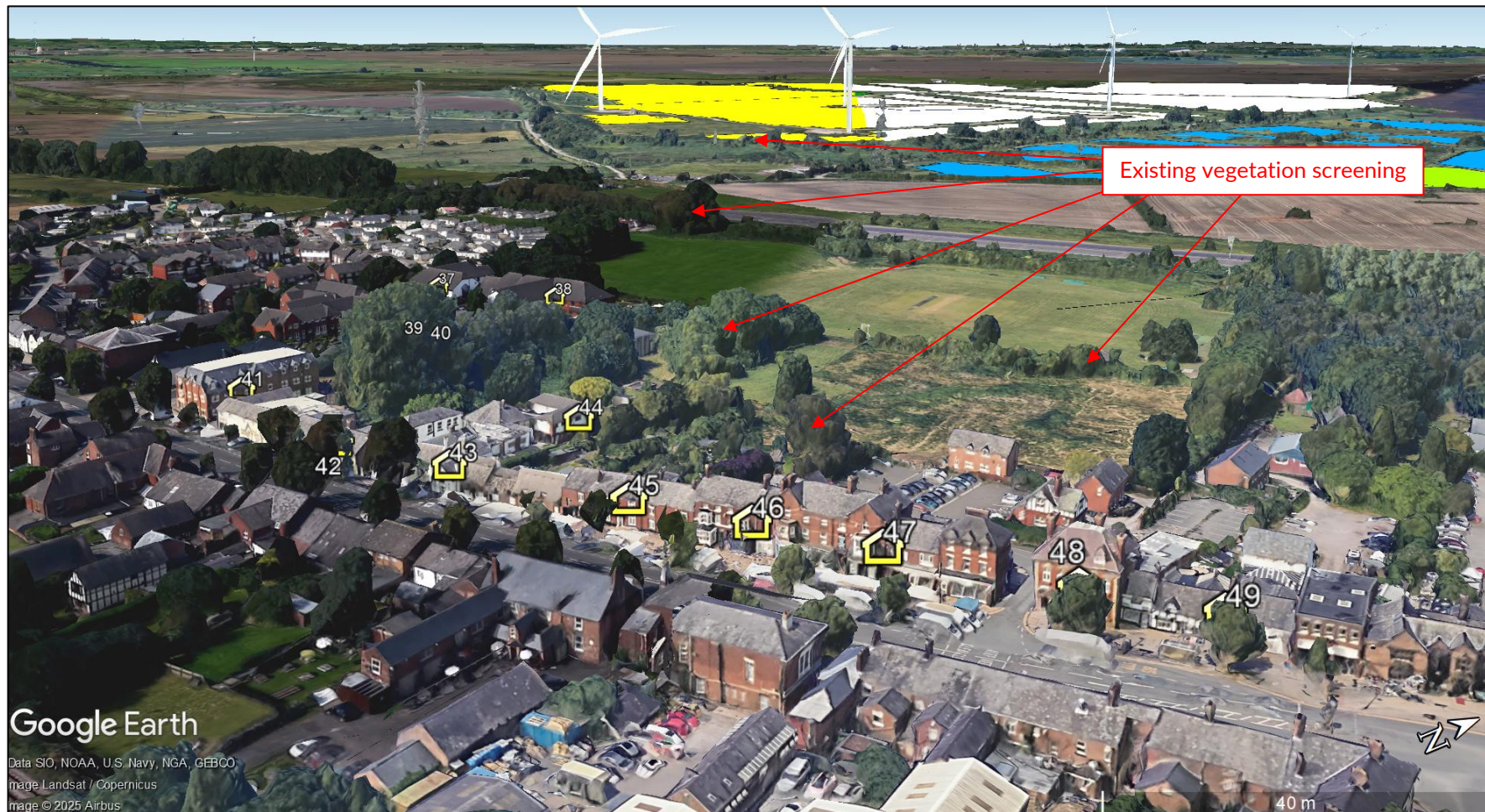
Figure J73 Reflecting panel areas and partial terrain screening for dwelling receptors 37 to 49
