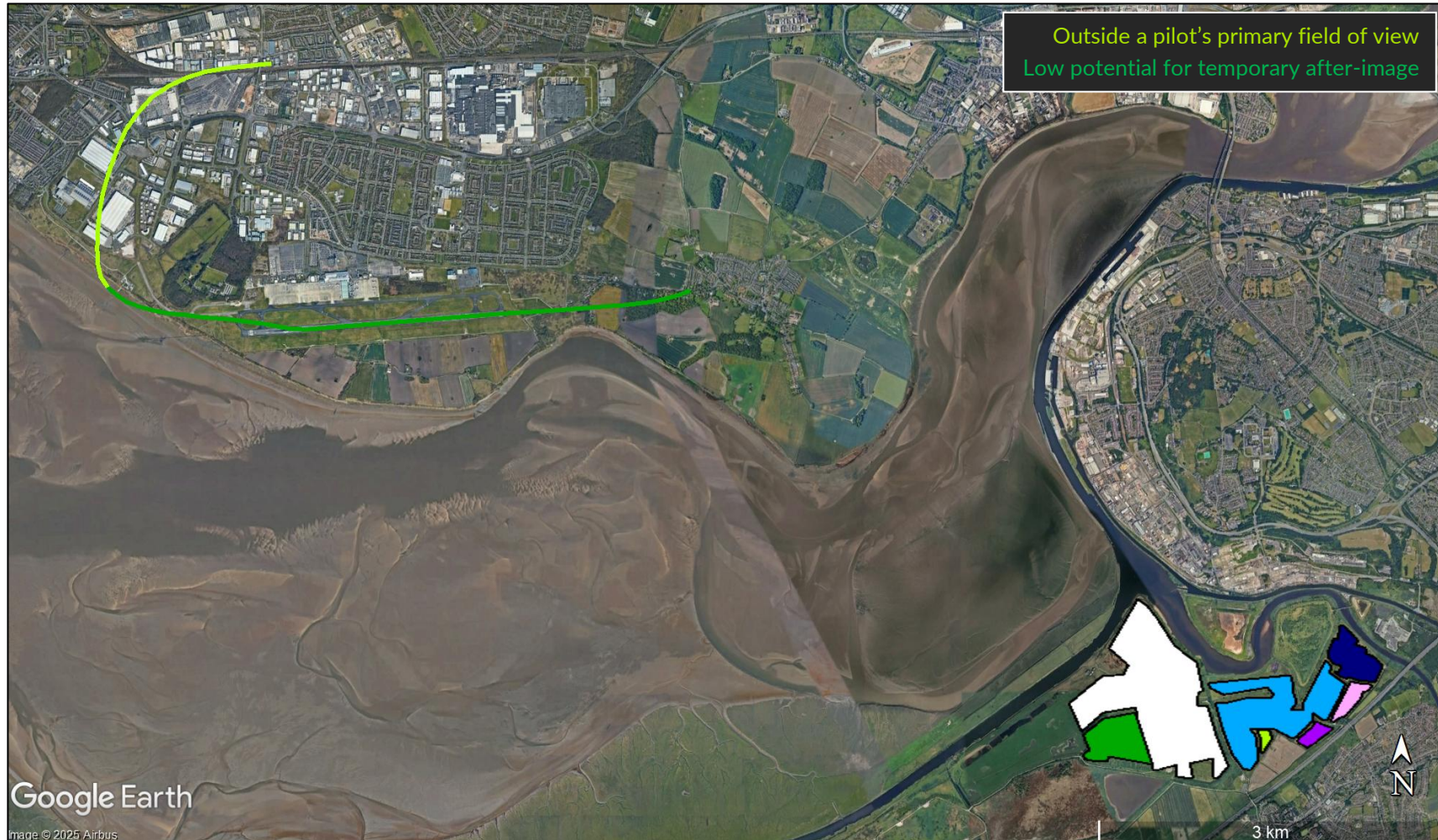
Figure 23 Solar reflections towards 09LH/ 27RH visual circuit
