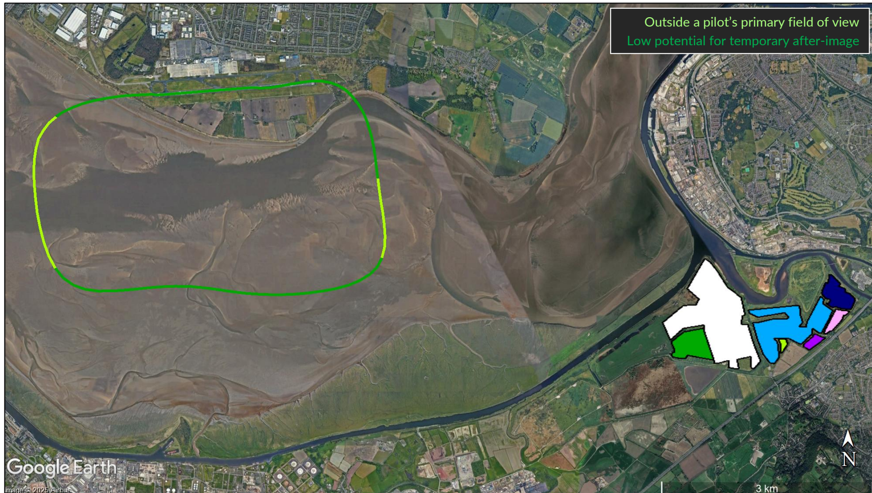
Figure 22 Solar reflections towards 09RH/27LH visual circuit
