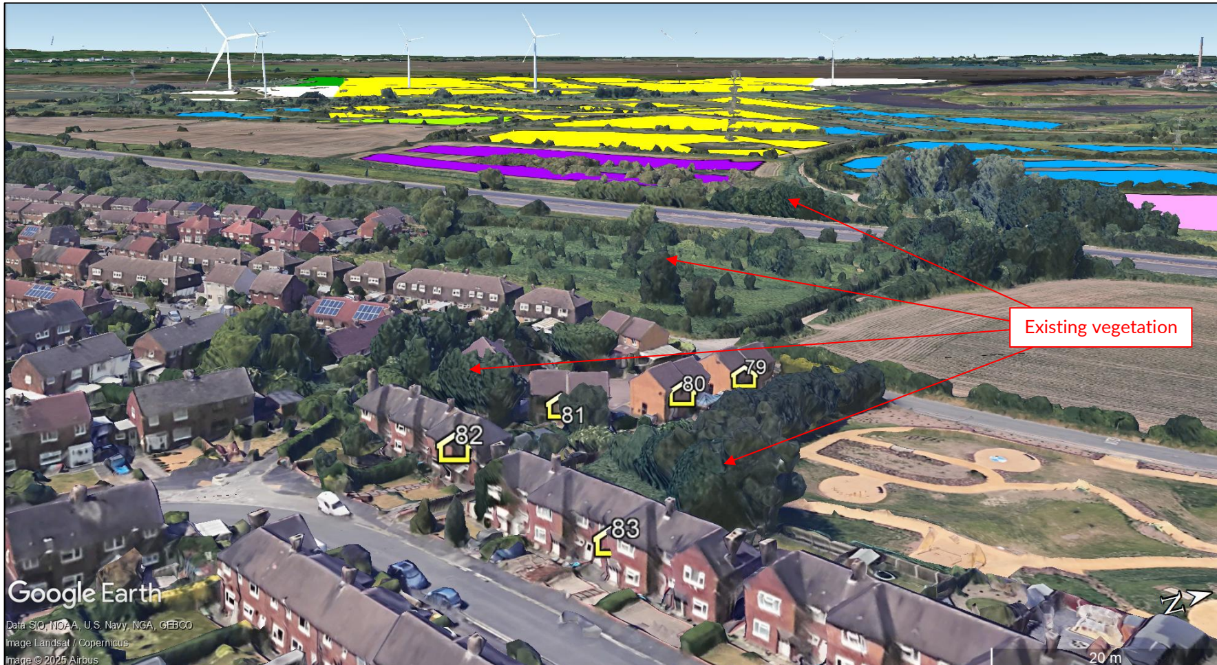
Figure J79 Reflecting panels and partial screening for dwelling receptors 79 to 83
