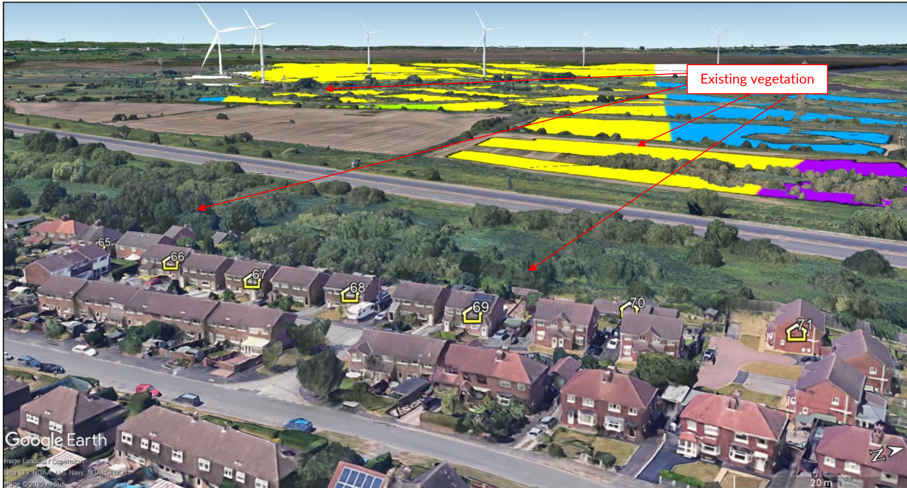
Figure J76 Reflecting panel area and partial screening for dwelling receptors 65 to 71
