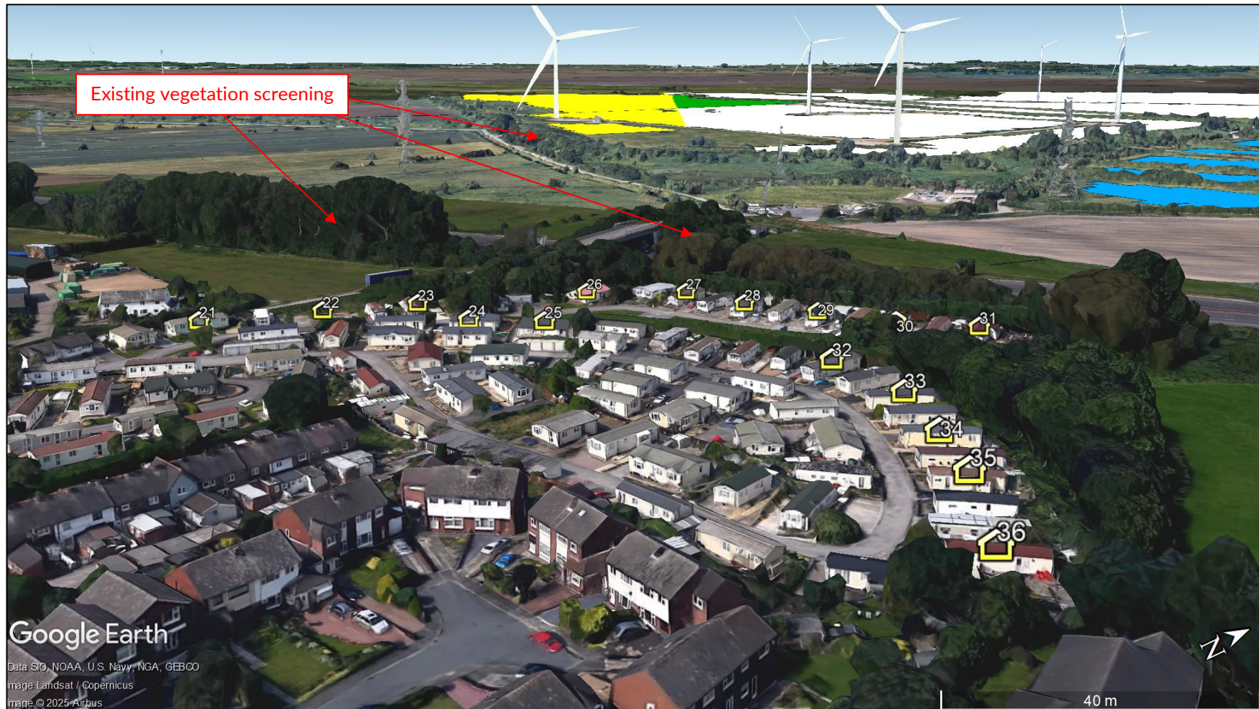
Figure J72 Reflecting panel areas and screening for dwelling receptors 21 to 36
